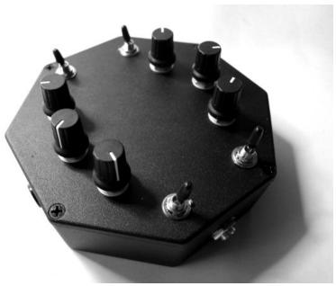
Power your Blackdeath with a BOSS-style 9v 2.1mm power supply. **IM-PORTANT:** +9v/positive on the outside, negative centre, minimum **200mA**). All orientation is with power socket on right/bottom (depending on model but it should be clear!). Jack input is top/left, output is on bottom/right.
