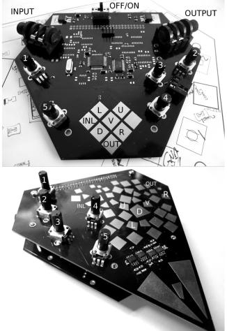
Describing each module, we refer to the knobs as numbered and the fingerboard directions Left, Right, Up, Down. See below - knobs effect U,D,R,L finger operations. INL and OUT refer to hardware routing (not so in Lachrymarum).
